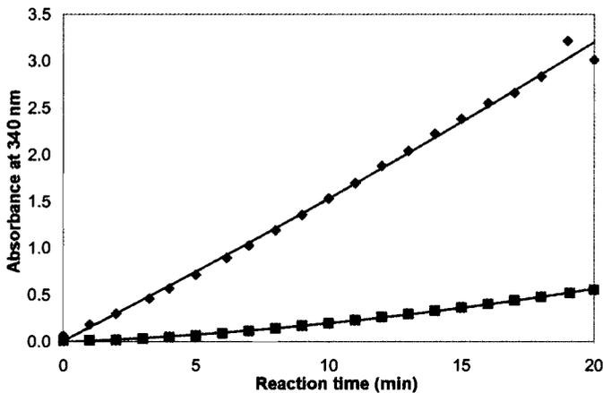
Fig. 2: Instability of MDH when the stock enzyme solution was prepared in phosphate buffer only with no added glycerol [15].  $\blacklozenge$  day 1;  $\blacksquare$  day 8
